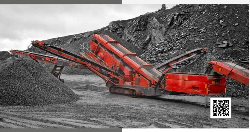
The Finlay® 696 2-deck inclined screen has been developed to fulfil the demands of high production producers in quarrying, mining, sand and gravel, coal, woodchip and topsoil applications.
