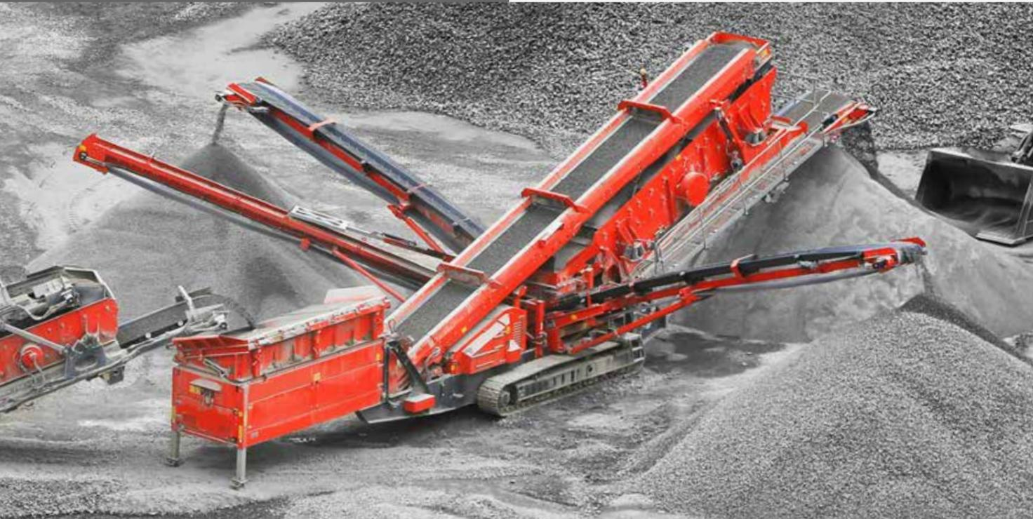
The Finlay® 696 3-deck inclined screen has been engineered to provide a superior high production solution in quarrying, mining, sand and gravel, coal, woodchip and topsoil applications.
