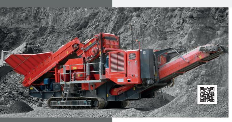
The Finlay<sup>®</sup> C-1540 hybrid mobile cone crusher offers operators the flexibility to power the plant either by mains electric <u>connection or the onboard genset powerpack configuration</u>.
