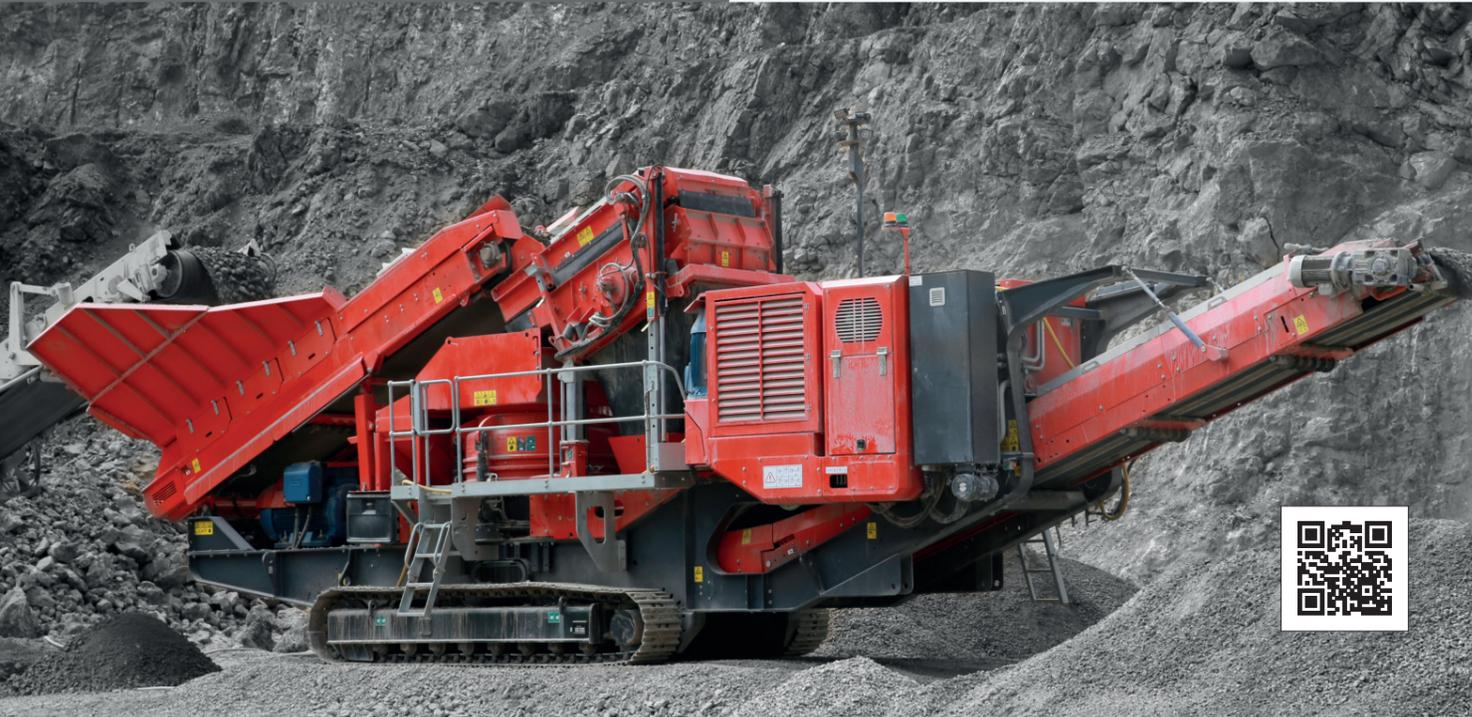
The Finlay® C-1540 hybrid mobile cone crusher offers operators the flexibility to power the plant either by mains electric connection or the onboard genset powerpack configuration.
