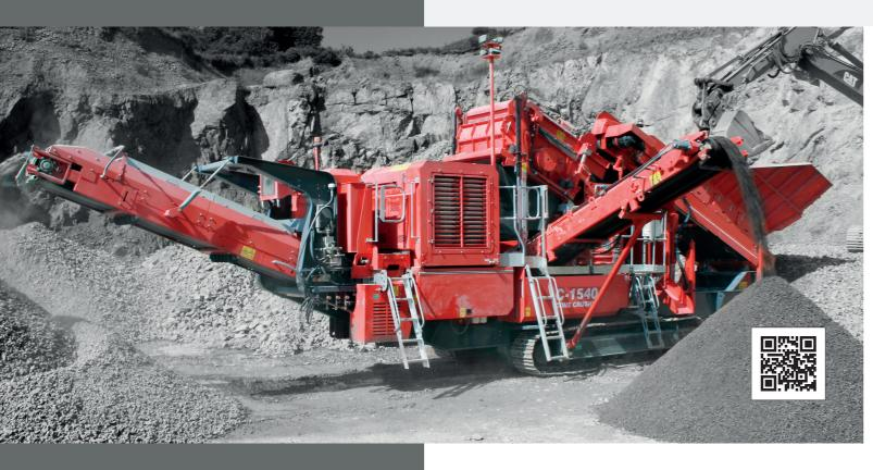
The Finlay® C-1540P mobile cone crusher has a proven pedigree in aggregate and ore surface mining applications. This efficient and productive machine incorporates the proven Terex® 1000 cone crusher with direct variable hydrostatic drive, automatic tramp relief and hyraulic closed side setting (CSS) adjustment.
