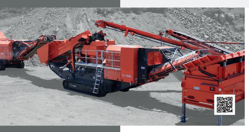
The Finlay® C-1545 is a high capacity and aggressive mobile cone crusher that consistently provides high output capacity and a product with excellent cubicity.
